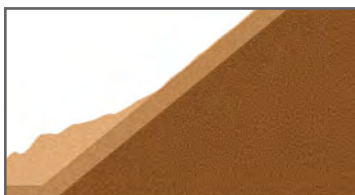
SHALLOW PLANE FAILURE
