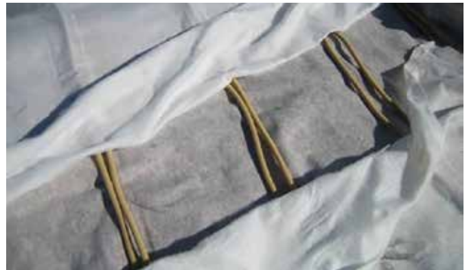
Figure 5: Transverse connections without couplers
