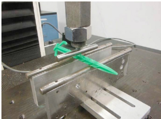
Bend Test Setup
