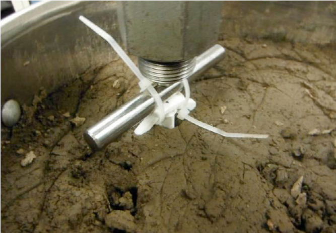
Pull Test - Sample Inserted
