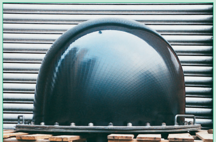
Fig. 8: Burst test of a Carbofol® according to EN 14151
