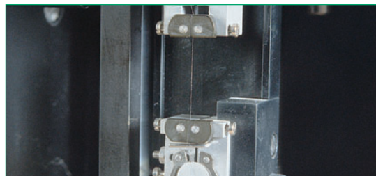
Determination of the strength and elongation properties of single fibres
